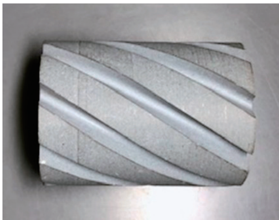
Fig. 5 Appearance of dry-machined SSNB3 ceramics.
