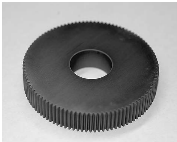
Fig. 3 Appearance of electrical discharge machined SAN-3 ceramics.
