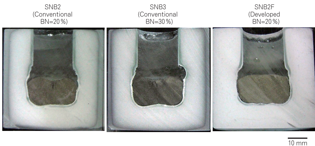
Fig.3 Cut surface of SNB series sample after corrosion test with molten metal. The photo on the left shows SNB2 with conventional 20% BN, on the middle SNB3 with conventional 30% BN, and on the right SNB2F with 20% ultra-fine BN.
